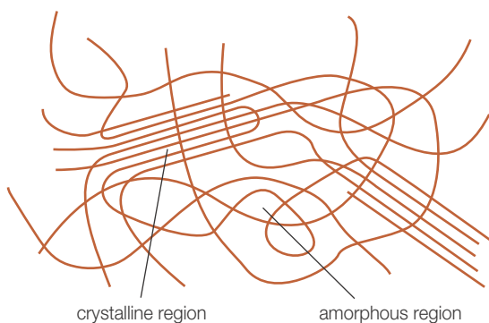
Figure 22.35 Crystalline and amorphous regions of a polymer
