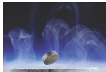
Figure 22.57 The Meissner effect: the floating magnet is only in contact with air
