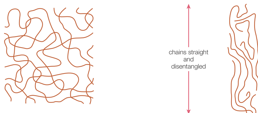
Figure 22.34 Unstretched and stretched rubber chains
